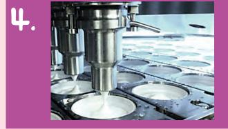
For fruit-on-the-bottom flavors, fruit is dispensed into the cups before the yogurt is added. The cups are sealed with foils and coded before being packed into
