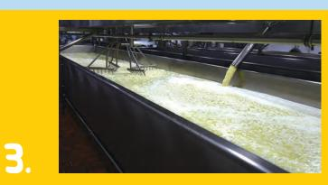
A special enzyme called rennet is added to the milk, which helps the "good" bacteria cause a chemical reaction that separates the milk proteins into liquids (whey) and solids (curds).
