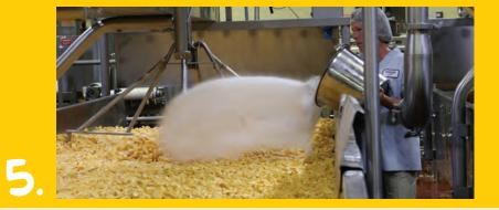
Salt and other ingredients for specialty cheese are added to the curds. Machines pack the curds into large blocks of cheese, which are then aged in a temperature-controlled warehouse.
